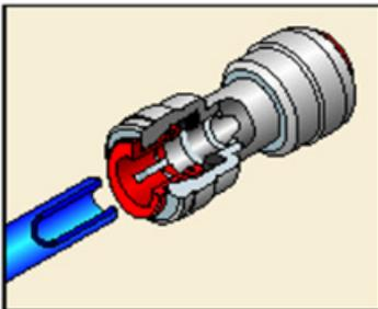
Insert the tube firmly until the tube end hits a positive stop.
