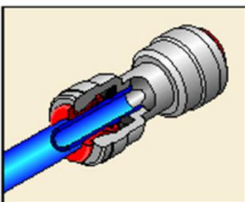
To check for a secure connection, tug on the tube with moderate force. The tube should hold in place. A stainless steel gripper ring holds the tube into the fitting and prevents o-ring leakage.
