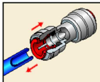
The unique oval-shaped face of the collets facilitates servicing. The wide oval shape allows easier finger placement for easy connecting and disconnecting.
