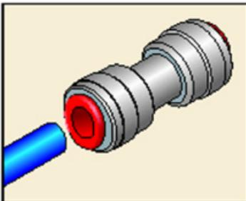
Cut the front end of the tube squarely before inserting. The outer surface of the tube end must be smooth, clean, and free from burrs and scratches.
